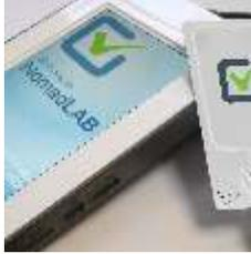
NomadLAB also supports **ISO7816** and **SWP** (HCI, HDLC) protocols for testing both contact smart cards, USIM cards and the contactless front end of NFC mobile phones.
